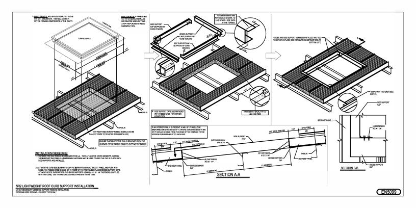
lssued : 06.01.20 (2020.012) **CERTIFIED ERECTION DETAILS** Detail Size (W x H) : 4 x 2
